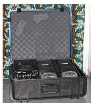
The radio station in a suitcase made by the company Wantok consists of an FM transmitter, a mixing desk, two tape recorders, two CD players, two microphones, headphones and cables. That's enough to run a village radio station.
