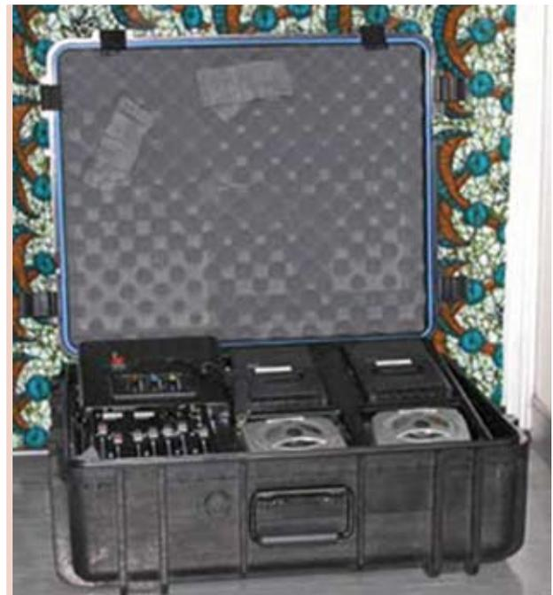
The radio station in a suitcase made by the company Wantok consists of an FM transmitter, a mixing desk, two tape recorders, two CD players, two microphones, headphones and cables. That's enough to run a village radio station.
