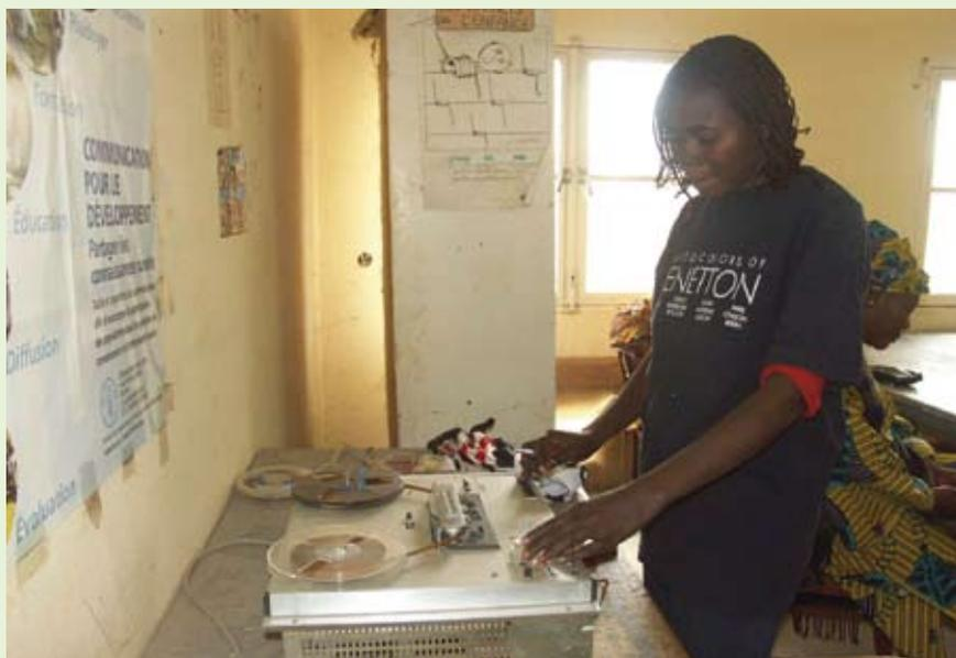
*The cutting of a radio batch using scissors on a magnetic tape recorder (above) – many of these have been used for more than 20 years*
